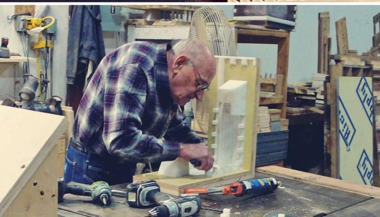
With more than a half-century's experience in cast stone and masonry production, Eugene Castonguay anchored Stone & Lime's Sharp Center textile block contract. A switch to the Teflon-coated plastic inserts and wet cast process boosted quality after he and colleagues started with wood inserts and a dry casting regimen.
